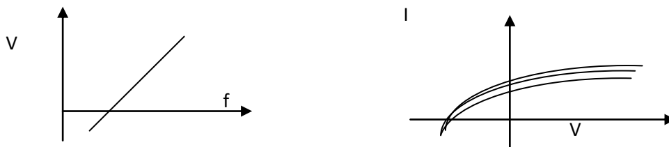
Figure 3: Stopping potential V vs f Figure 4: Current (Intensity) vs retarding and accelerating V
