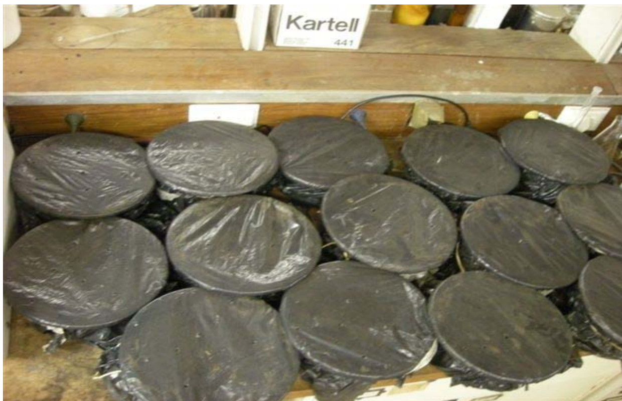
Fig. 2.0. The co-compost piles of oil sludge, soil, wood chips and animal manures incubated under laboratory conditions.
