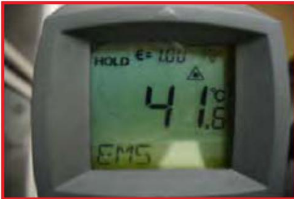
Figure 3.7: Simulation of an IR Thermometer measurement reading at \epsilon=1.00 [22].
