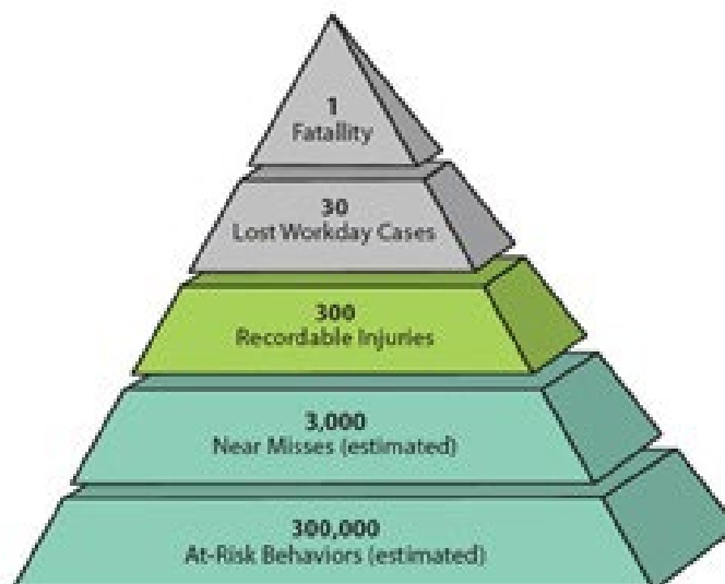
Figure 5: ConocoPhillips Marine safety pyramid (Source: Rockwell Automation, 2007)
