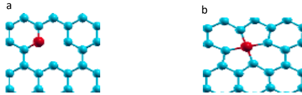
Figure 6.5: (a) Pre-relaxed (b) relaxed structure of silicene containing nearest-neighbour vacancy-vanadium defect complex, v0-Vs1 . The blue spheres represent the silicene atoms, while the red sphere represent the vanadium atom.
