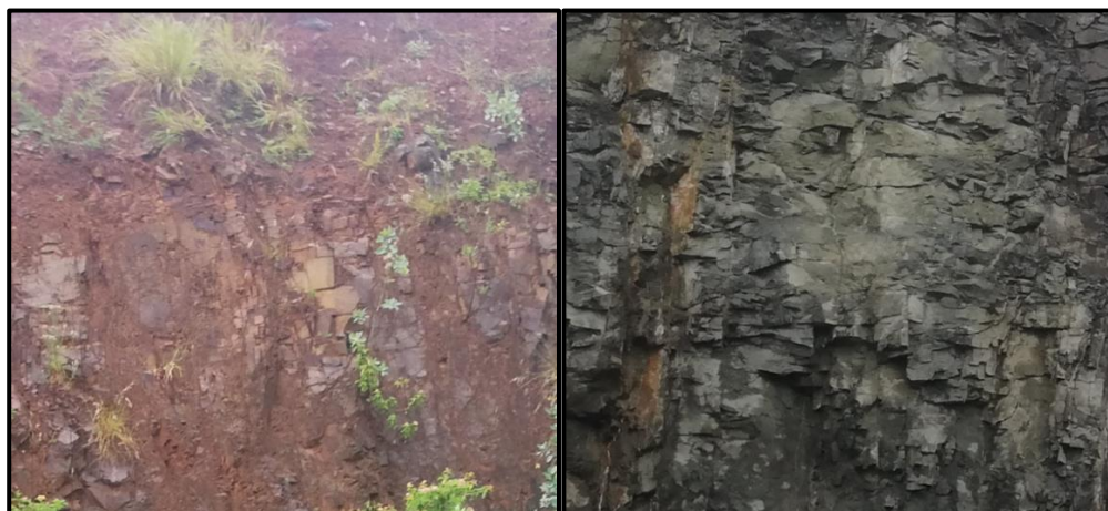
Figure 3.3: Example of an unfavourable site (on the left) and a favourable site (on the right) for face mapping.
