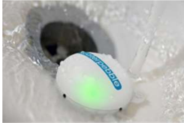
Figure 5: A Water Pebble used to monitor the amount of water used. Source: Scarfiello (2015)
