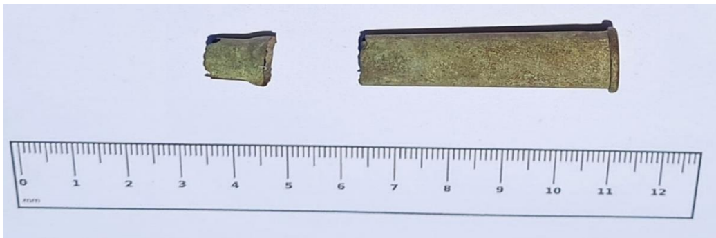
Figure 35: .303 cartridge with its front part neatly cut off
