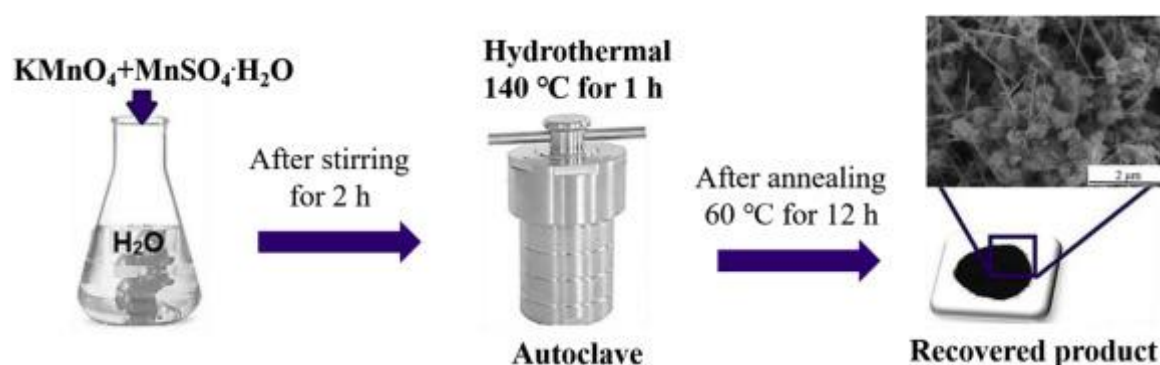
Figure 2.5: Schematic representation for the synthesis of \text{MnO}_2 using hydrothermal method. Reprinted with permission [39].
