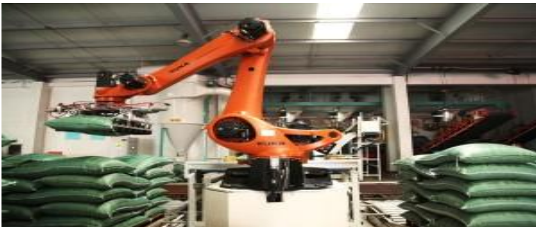
Figure 4.1: A representation of a stacking Kuka Robotic used at VW that is referred to by the participant.
