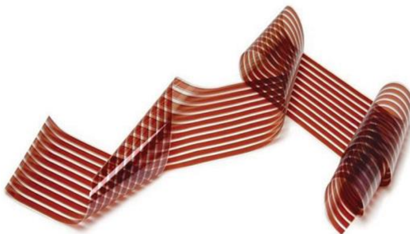
Figure 2. 6: Organic solar cell cast on a flexible substrate. It can be stretched, rolled or even curved in any direction [26].
