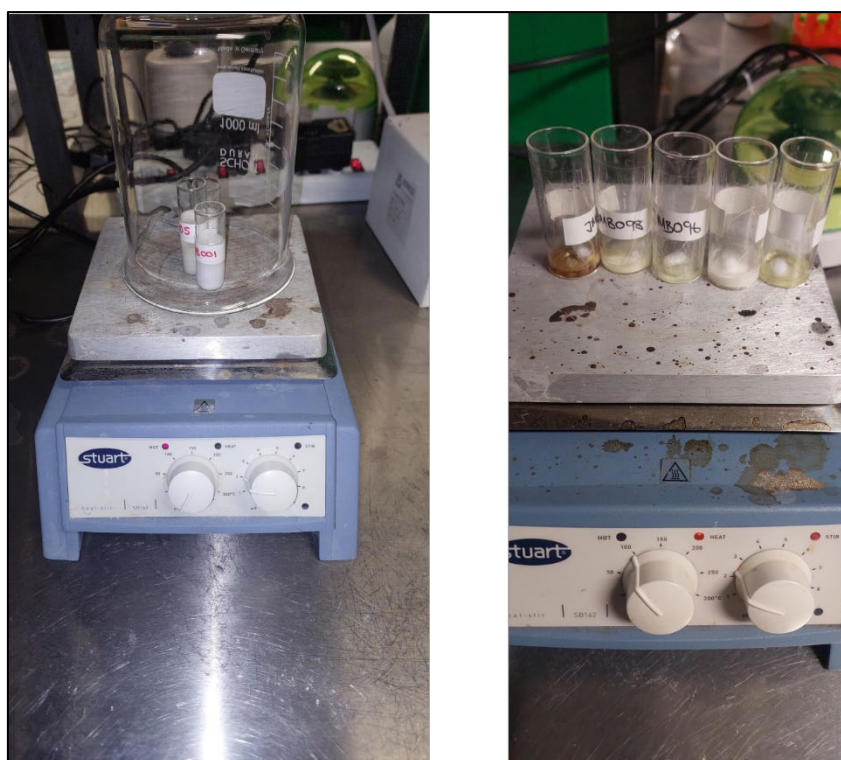
Figure 3. 1 Setup of hotplate and polytop vials for dissolving the starting materials
