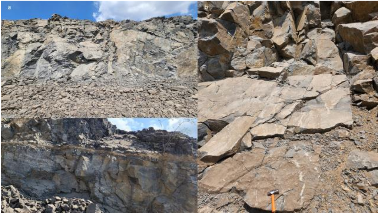
FIGURE 4.2: JOINT ORIENTATIONS FOUND AT THE OPEN-PIT MINE. (A) OPEN JOINTS THAT LOOK LIKE SLOPE FACE ON THE WESTERN PART OF THE OPEN MINE PIT, (B) 3 SET OF JOINTS ON THE WESTERN PART OF THE OPEN MINE PIT AND (C) OPEN AND CLEAN JOINTS ON THE NORTHERN SIDE OF THE PIT.
