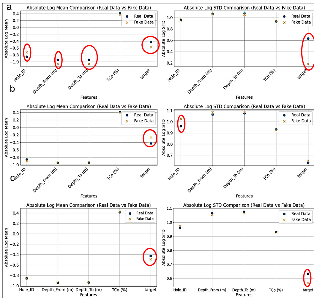
Figure 4.6: Mean and standard deviation of real and fake for assay data: a) CTGAN; b) CopulaGAN; and c) GaussianCopula
