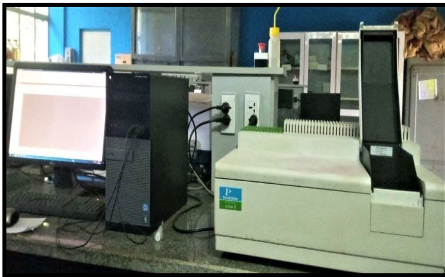
Figure 6.1: A Figure showing UV-Vis spectroscopy.
