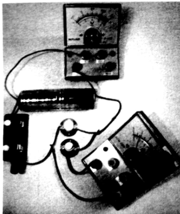
Figure 1 Apparatus set up for the practical activity (measuring V_p and I_2 ).
