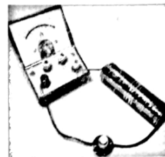
Figure 2 An ammeter connected in series in a circuit.
