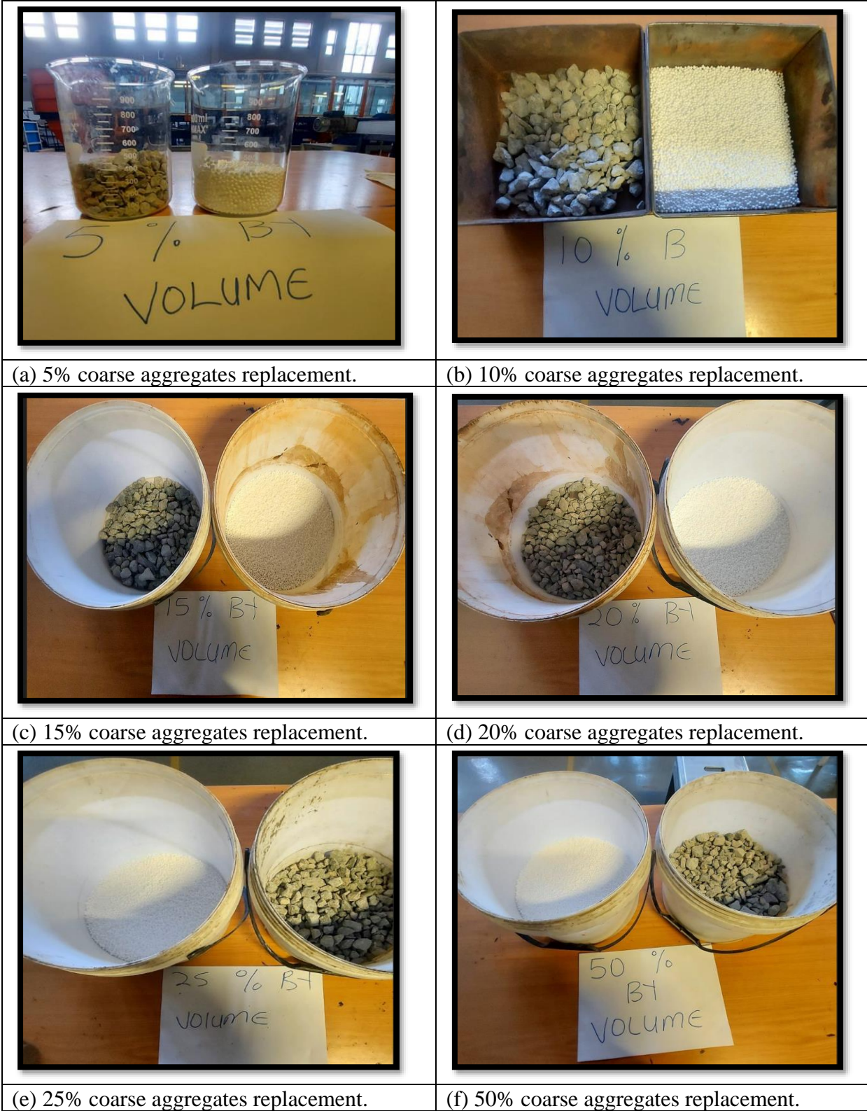
Figure 3-2: Measured Equivalent EPT Volume Used to Replace Coarse Aggregates
