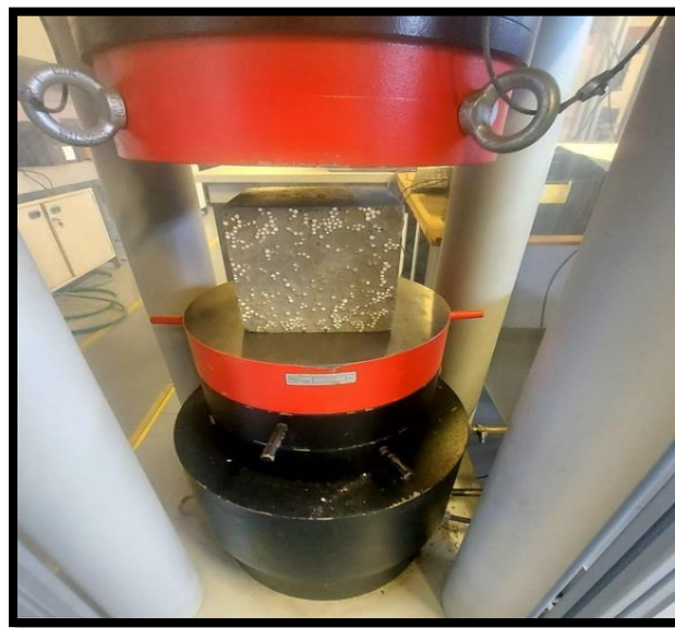
Figure 3-3: Compressive Strength Test Setup
