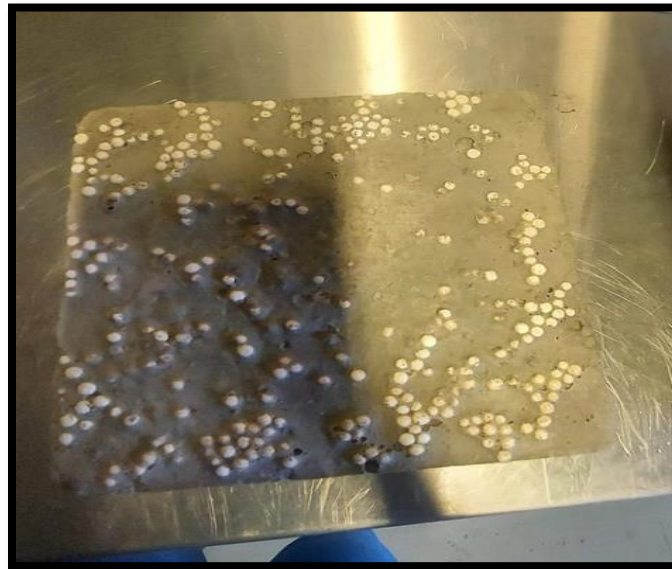
Figure 4-3: EPT Beads Escaping to The Surface
