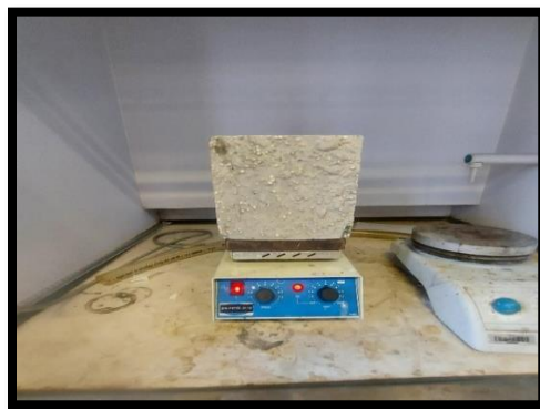
Figure 3-6: Heat Conductivity Test Setup
