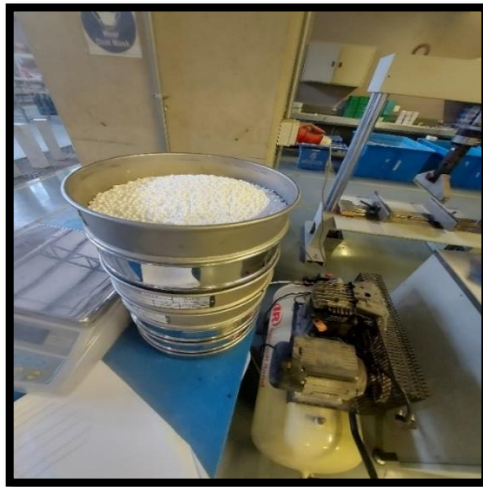
Figure 3-1: Illustration of Particle Size Distribution Test on EPT
