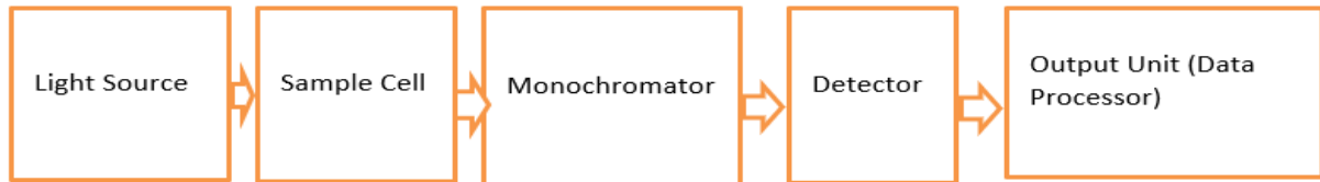
Figure 3.4: Schematic flow diagram of Atomic Absorption Spectrometry (AAS) used to analyze toxicity of ion within metals (Researcher, 2019).
