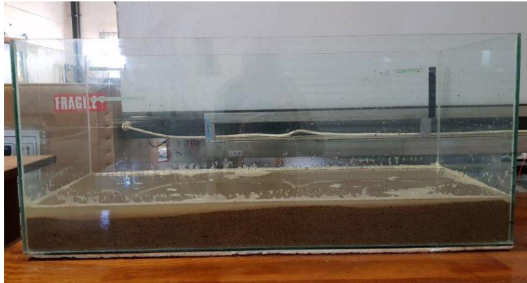
Figure 3-4: A 7-day inoculation of biological activated sand (BAS) set-up (picture taken by S Sambo, 2019)
