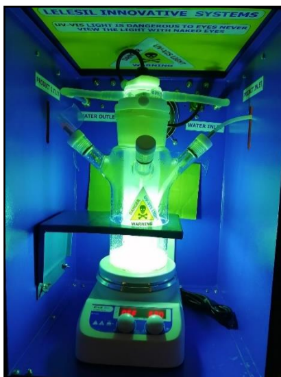
Figure 3. 3: Photoreactor used for the photocatalysis and photocatalysis-coagulation experiments.
