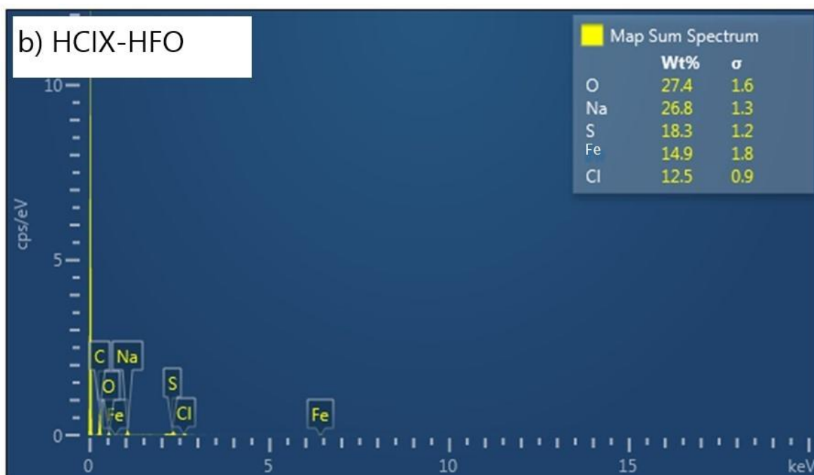
Figure 4.2: b) EDS spectra of cross section HCIX-HFO resin bead.
