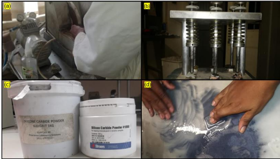
Figure 3.7: Thin section preparation at the laboratory. (a) Cutting machine, (b) Drying process, (c) Course and fine silicon carbide powder, and (d) Polishing
