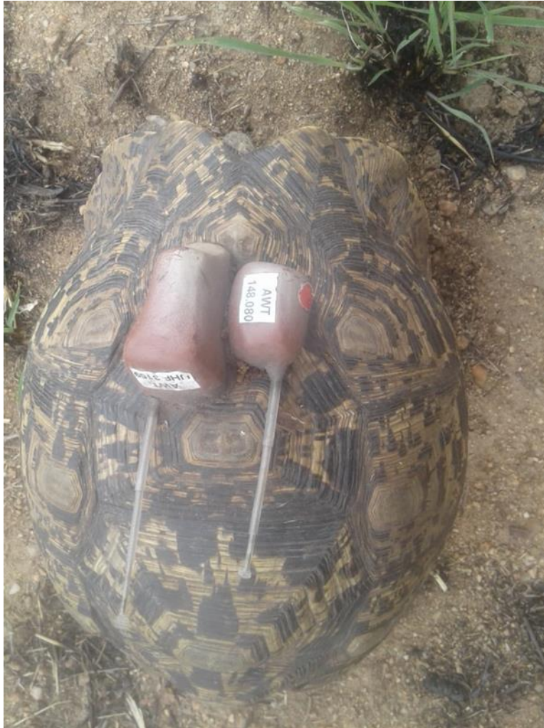
Figure 4.1. A leopard tortoise ( Stigmochelys pardalis ) fitted with VHF and UHF transmitters for tracking and GPS data collection respectively.
