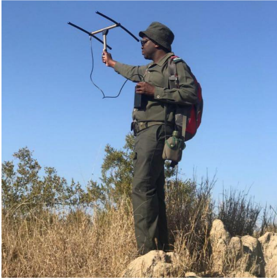
Figure 4.2. The researcher locating tortoises in the field with a four element Yagis antenna and Communications Specialists Inc. receiver.
