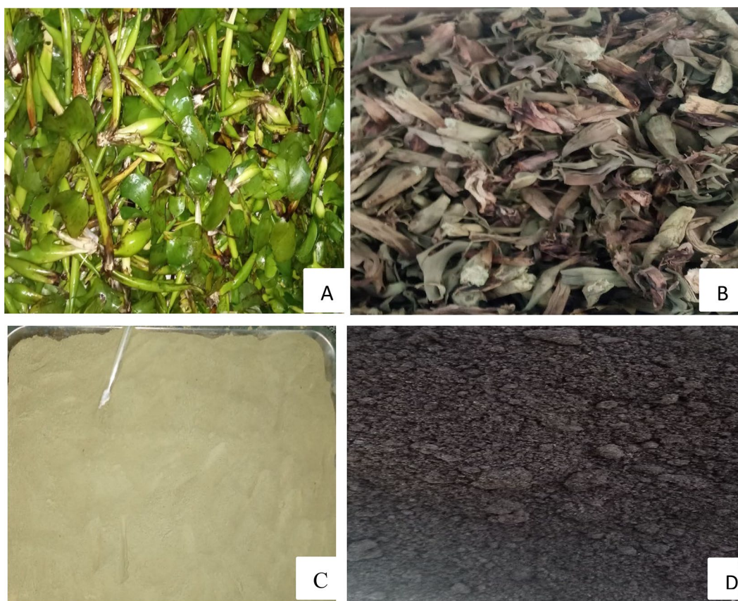
Fig. 1 The different stages of AC preparation A–D . Where ‘ A ’ indicates the raw Erichornia crassipes , ‘ B ’ indicates the dried Erichornia crassipes , ‘ C ’ indicates the crushed Erichornia crassipes , and ‘ D ’ indicates the final product (AC)
