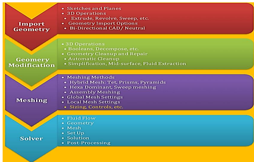
Figure 2.9: ANSYS Simulation workflow [21]
