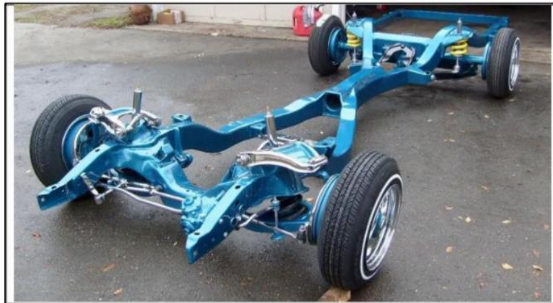
Figure 2.3: X frame chassis frame [12]
