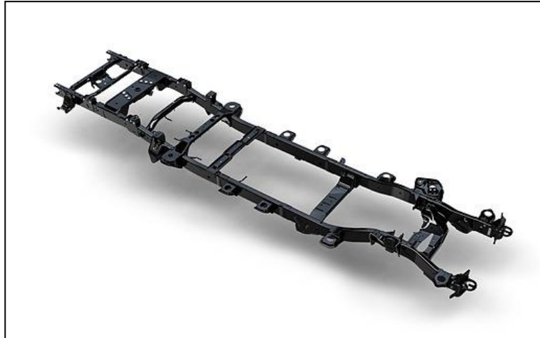
Figure 2.1: A ladder chassis frame [10]
