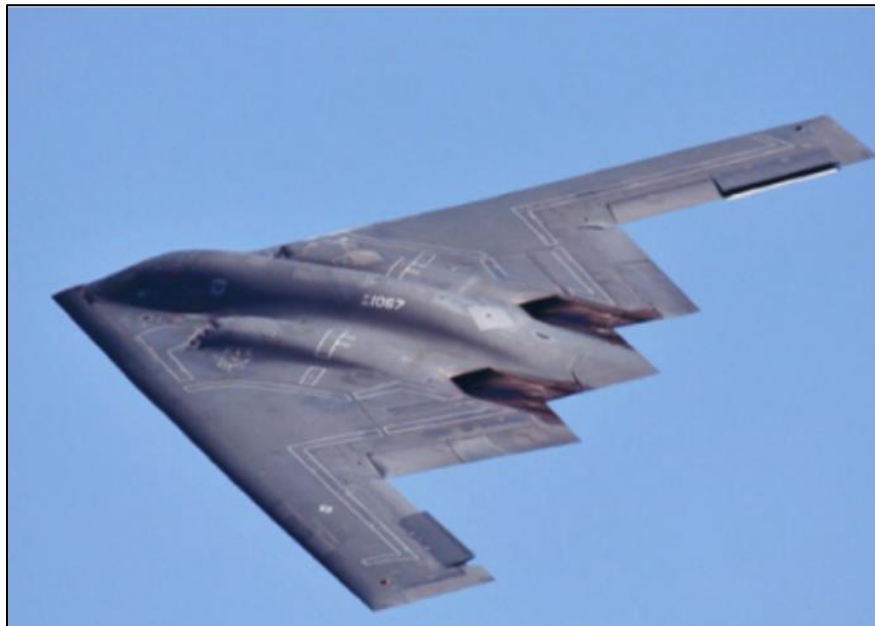
Figure 124: B-2 Bomber is microwave absorbing and primary radar invisible (Okonkwo and Smith. 2015).
