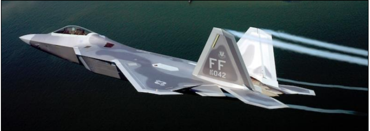
Figure 123: F-22 Raptor is microwave absorbent and thereby reduces its radar cross section considerably (USAAF. 2015).
