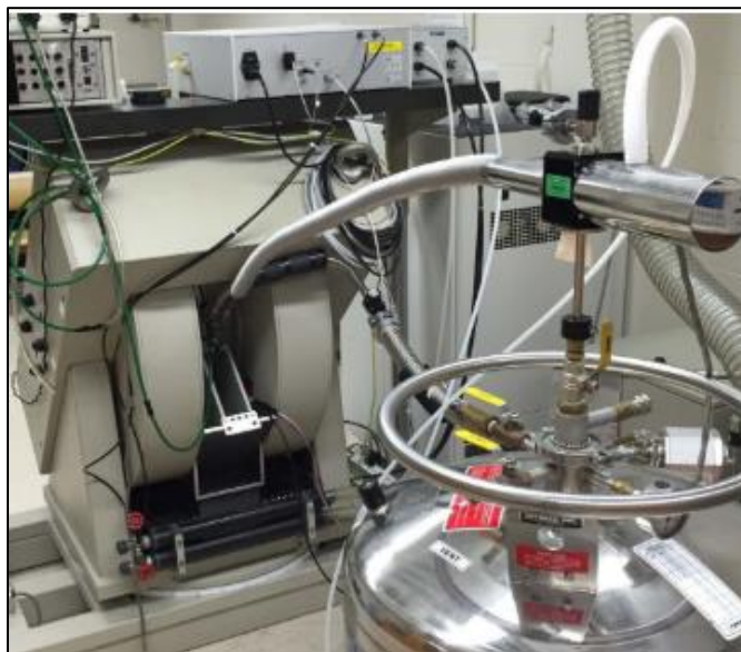
Figure 106: Illustration of liquid helium tank connection to a ESR900 Continuous flow Cryostat. < https://epr.chem.wisc.edu/content/instruments > [Accessed on 12 Jan 2020].
