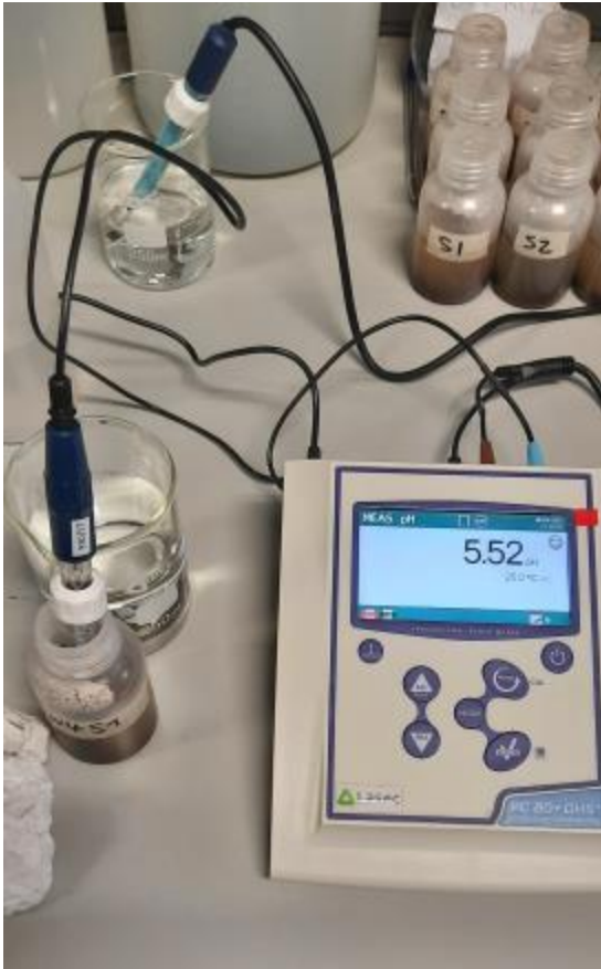
Figure 3.6: Electrode immersed into upper portion of solution (Kullander, E., Roodepoort, March 2021)
