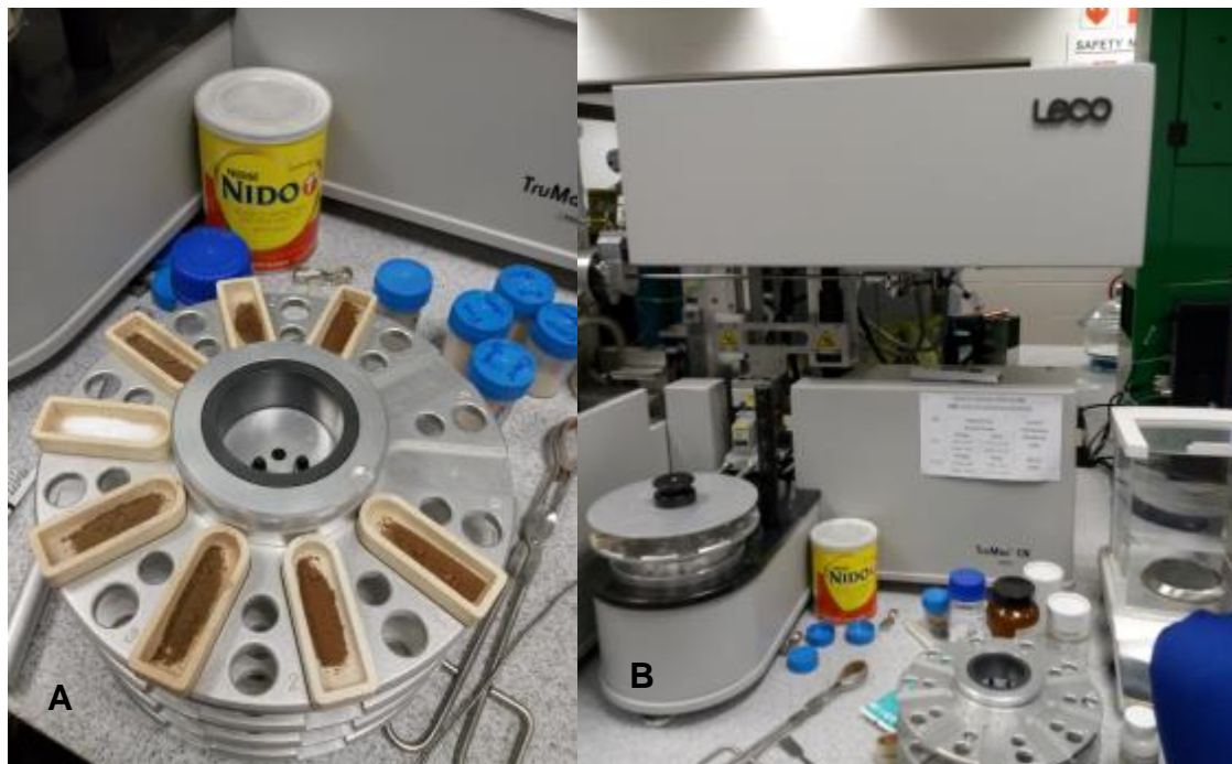
Figure 3.11: Ceramic boats containing soil samples (A) for analysis in the LECO analyser (B).
