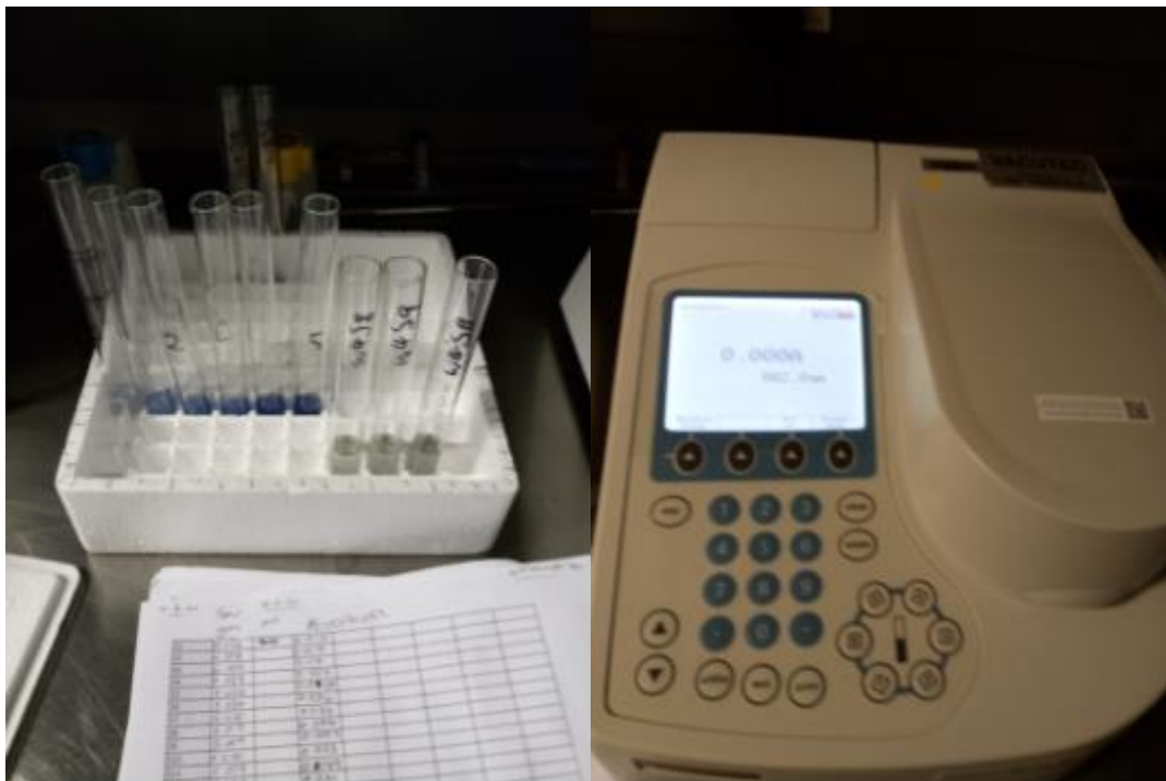
Figure 3.9: Standard series and soil sample solutions and spectrometer (Kullander, E., Roodepoort, March 2020)
