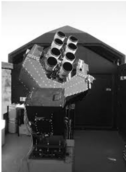
Figure 3.4: SuperWASP-S with its 8 Camera arrangement (Pollacco et al., 2006).
