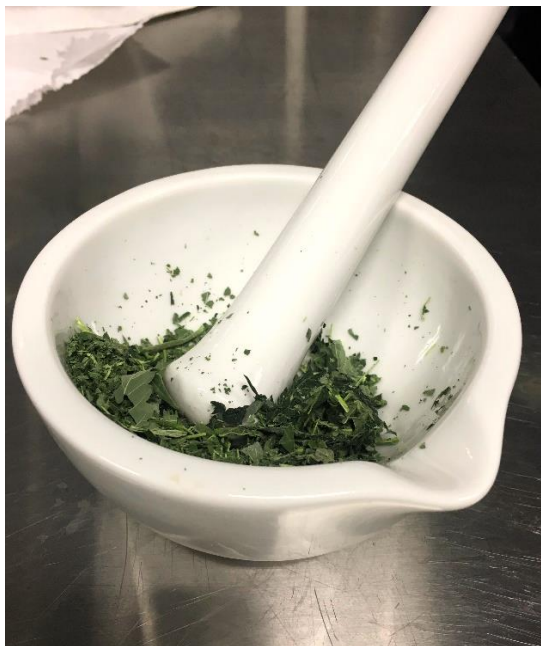
Figure 3.2a: Grinding freeze dried vegetative Cannabis leaves using a mortar and pestle. (Source: Pictures were taken during the process of investigation).
