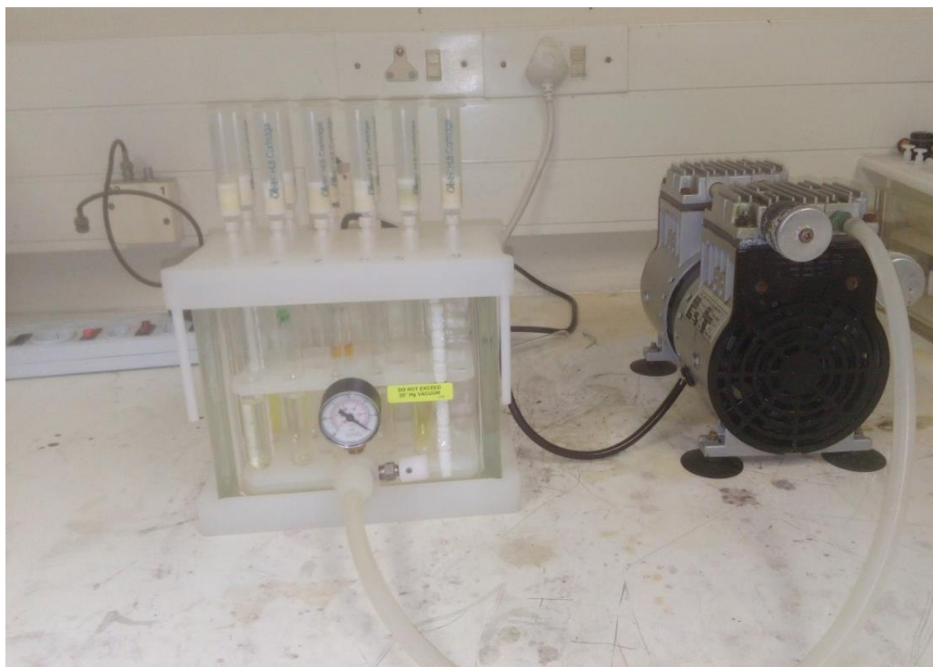
Figure 3-4: Manual solid-phase extraction setup used for the extraction of mycotoxins
