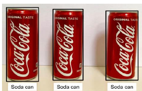
Figure 1.15: Multiple instances of the same object are detected by the same model trained to detect one object instance.
