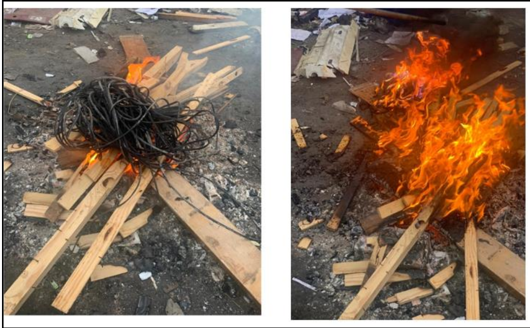
Figure 4.19: Open fire burning of cables at informal recycling centre in Umgeni Road, eThekweni (Source: Mkhwanazi, 2019)
