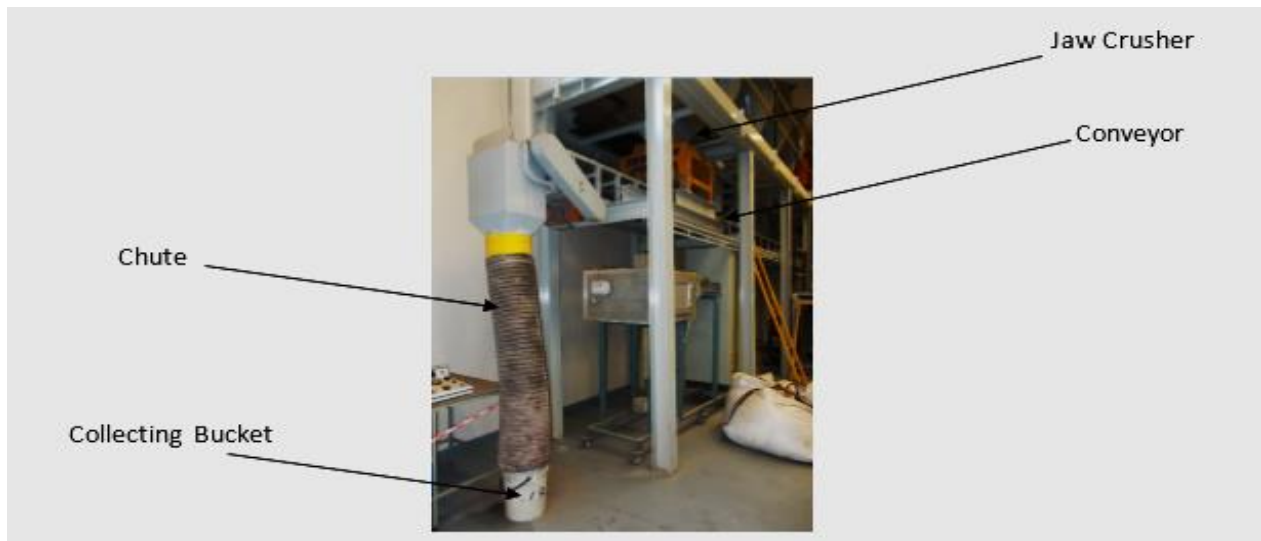
Figure 3.4: Jaw crushing circuit.
