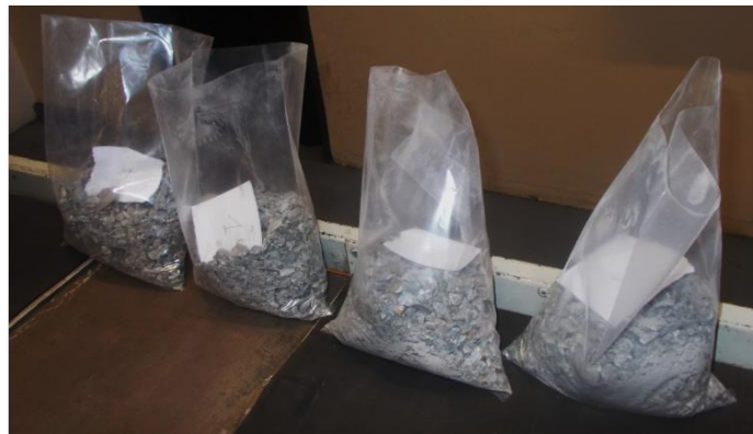
Figure 3.7: Samples of jaw crusher product after sieving.
