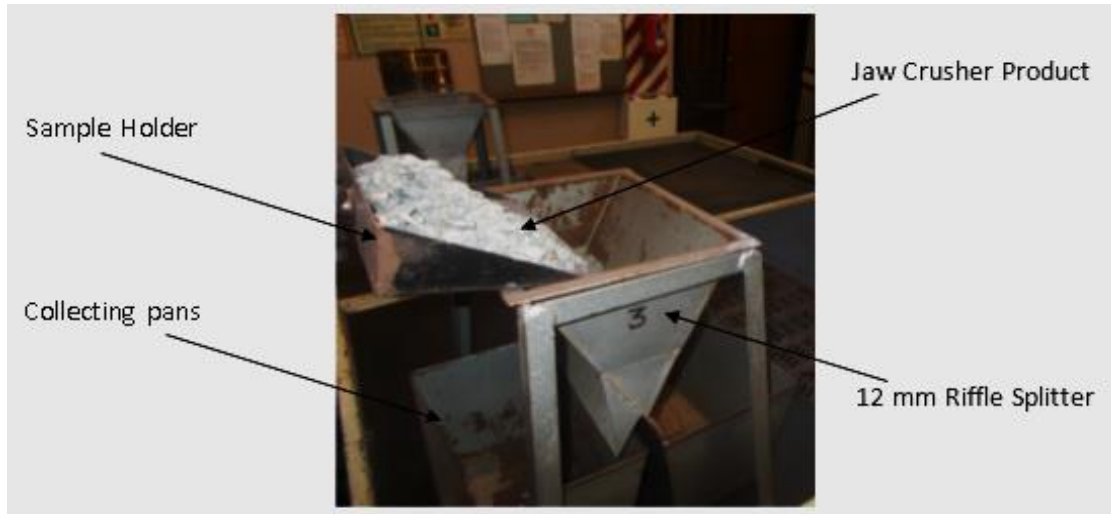
Figure 3.5: Splitting of jaw crusher product.
