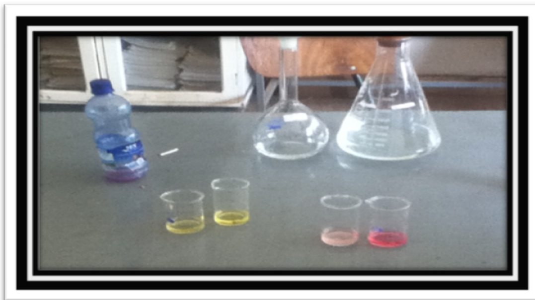
Figure 2.9 Comparison of water extract Indicator from a Red colored flower with industrially prepared methyl red in acid and base reaction.
