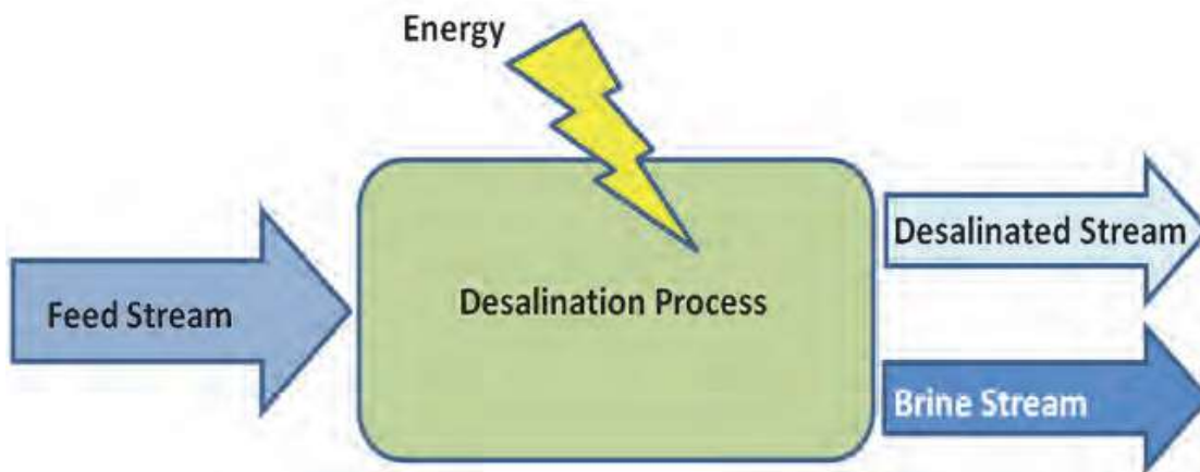
Figure 2: Schematic representation of the desalination process (Adapted from WRC Report No TT 637/15).
