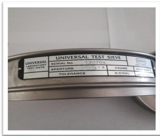
Figure 4: Universal test sieve 355 \mu m
