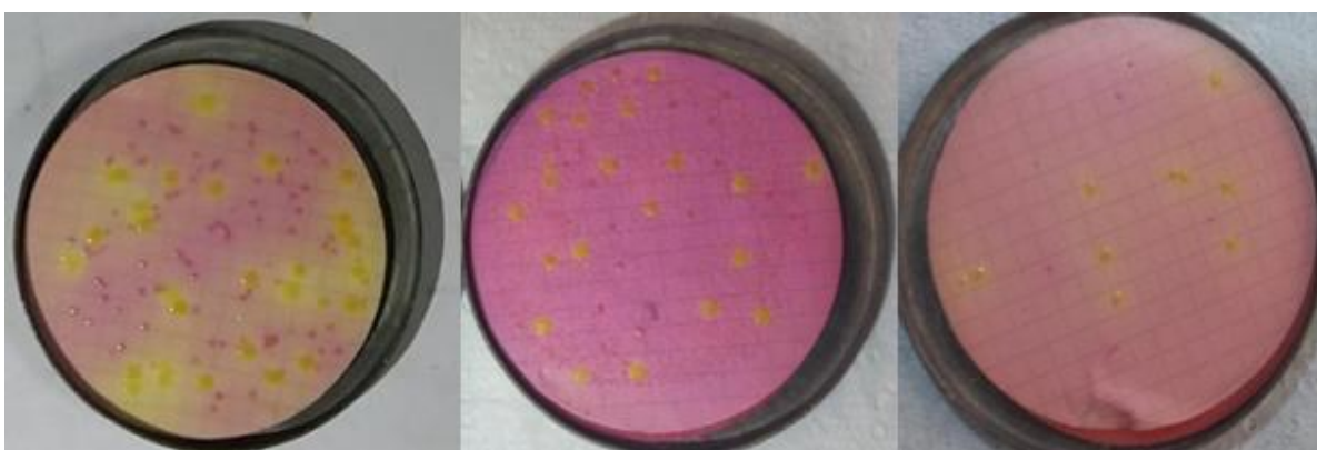
Figure 4.3: Sample of the thermotolerant coliform colonies test results
