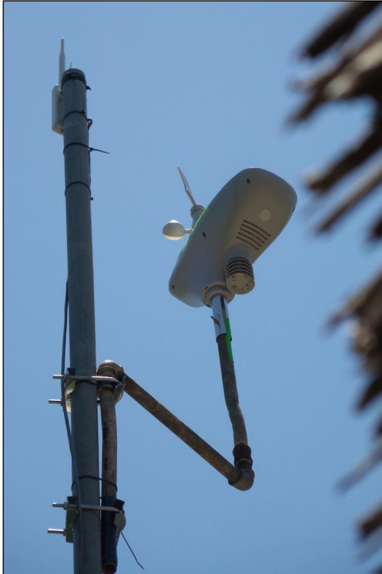
Figure 12-4: Ambient Weather WS-1000-WiFi OBSERVER Solar Powered Wireless Wi-Fi Weather Station mounted on an 8-meter-high mast.
