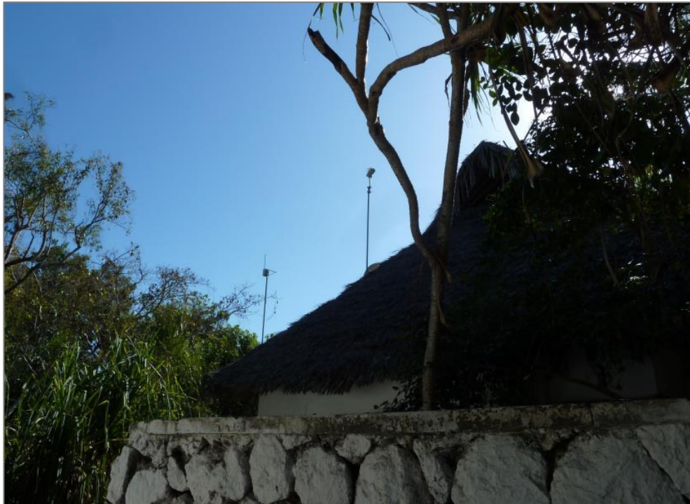
Figure 12-5: Weather Station mounted above the height of the office roof and clear of any obstructions.
