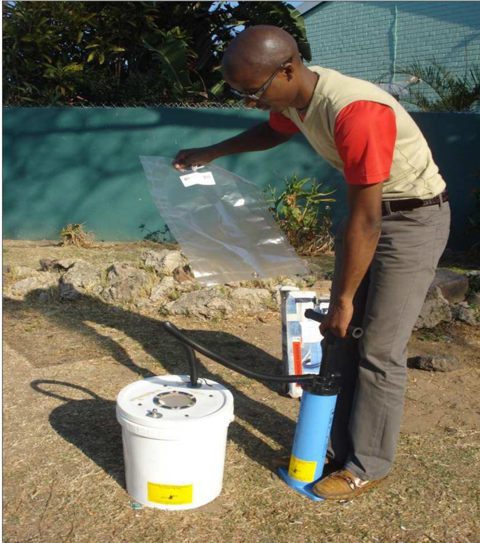
Figure 4.1: The Bucket Brigade sample setup and instruments used (SDCEA, 2012).
