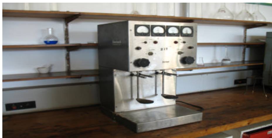
Figure 2: Electrochemical machine with 25 volts dc power
