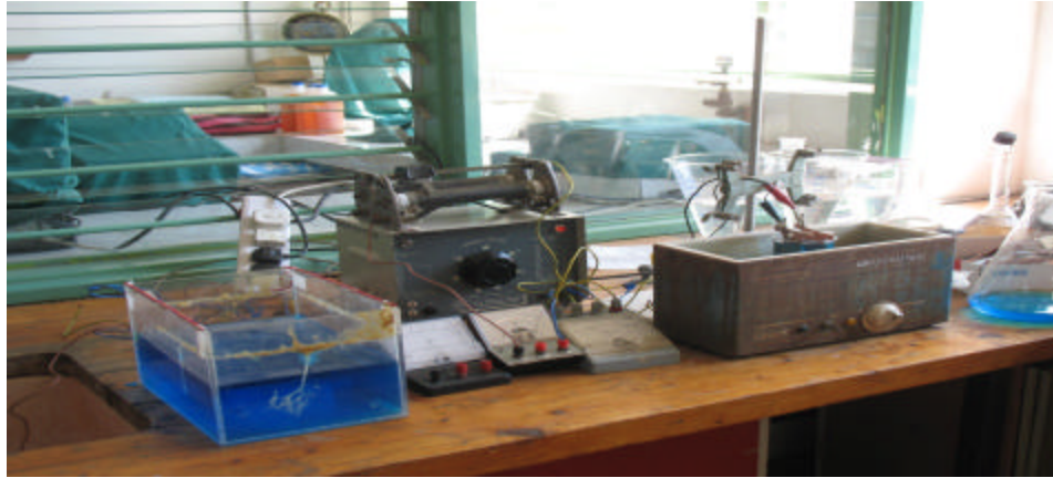
Figure 5: Batch reactor immersed in water bath
