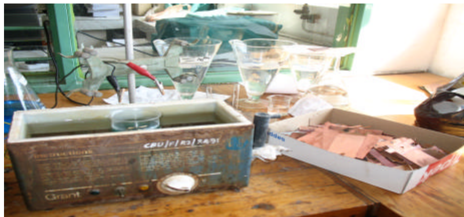
Figure 1: The thermostat controlled water bath and electrodes
