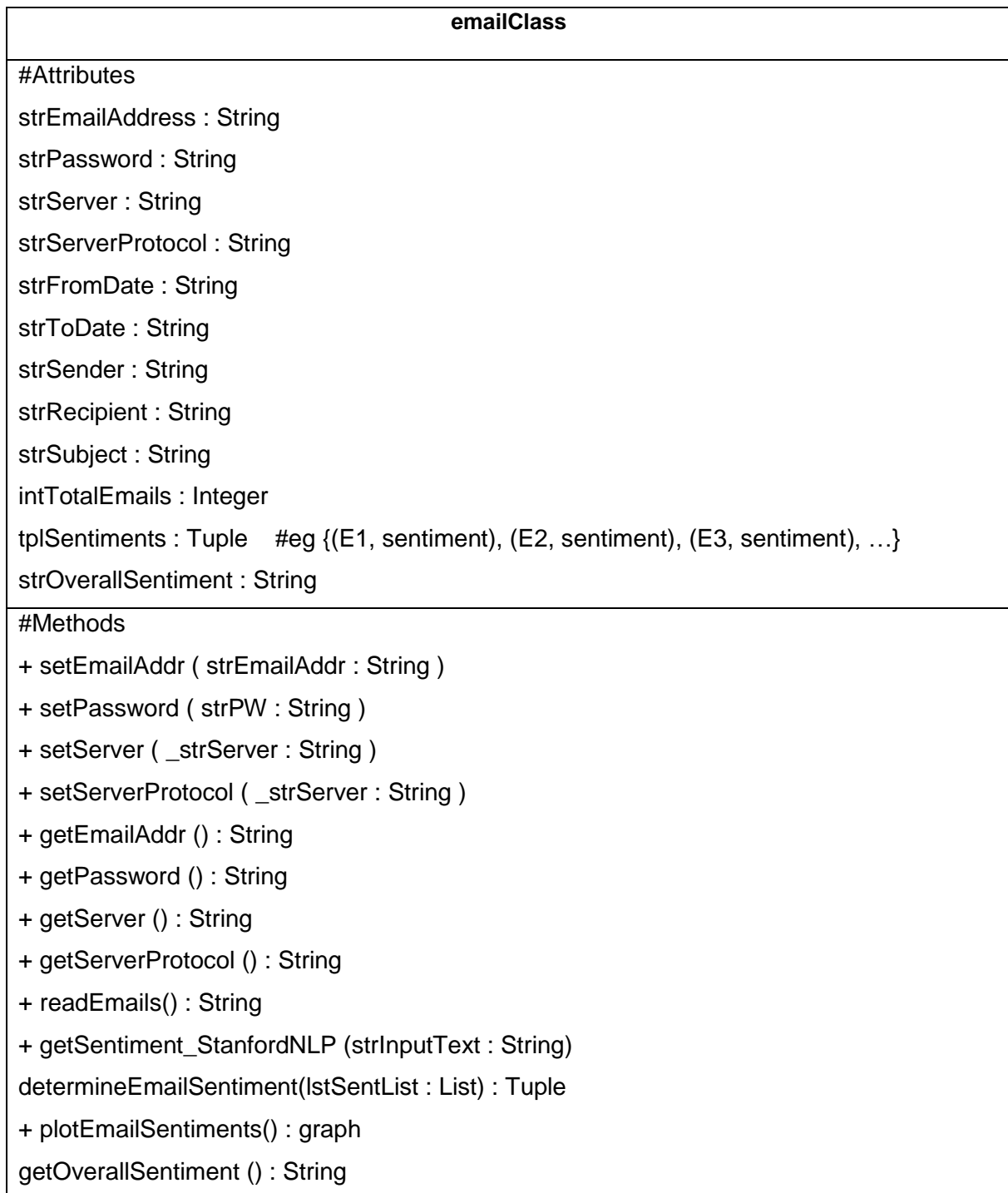
Figure 5.11 – Class diagram of the emailClass
