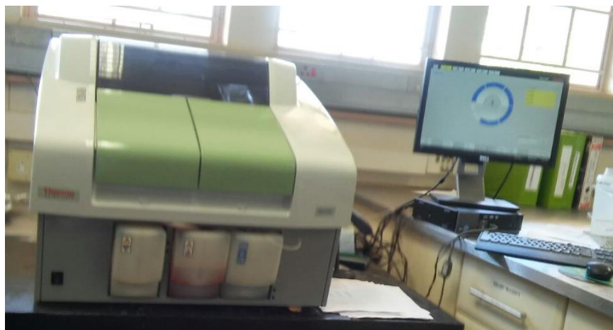
Figure 3-5: Bench top discrete analyser (Gallery instrument)
