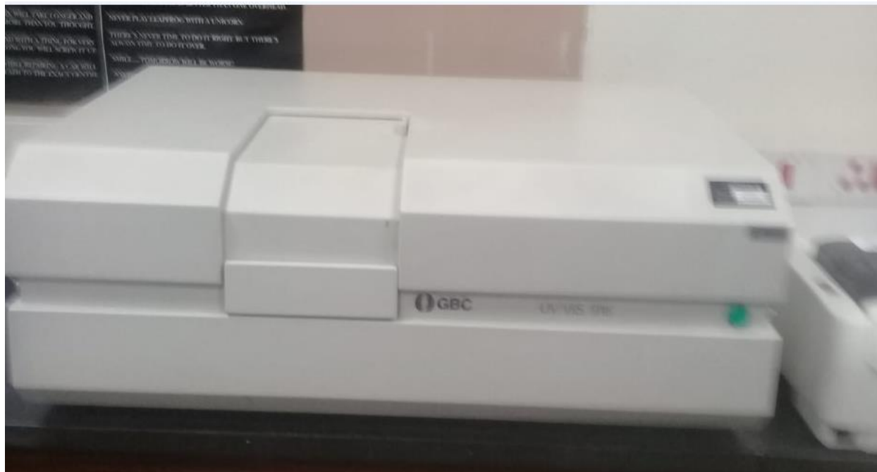
Figure 3-11: GBC-UV/VIS instrument for Chlorophyll analysis. Source: (Author).
