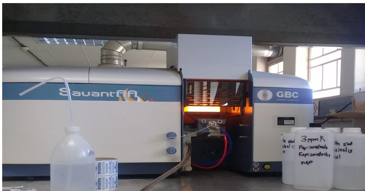
Figure 3-10: GBC Savanta Atomic Absorption Spectrometer (Source: Author)
