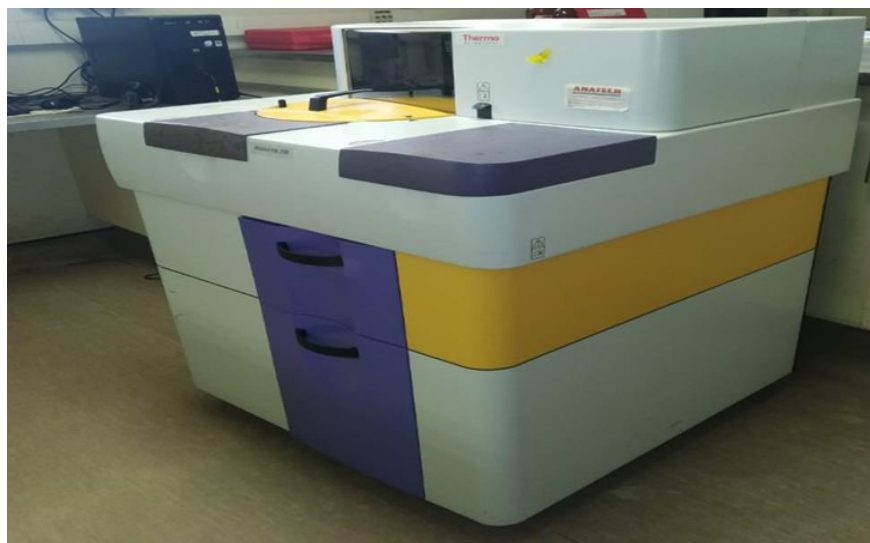
Figure 3-6: Discrete analyser that uses floor space (Aquakem instrument).
