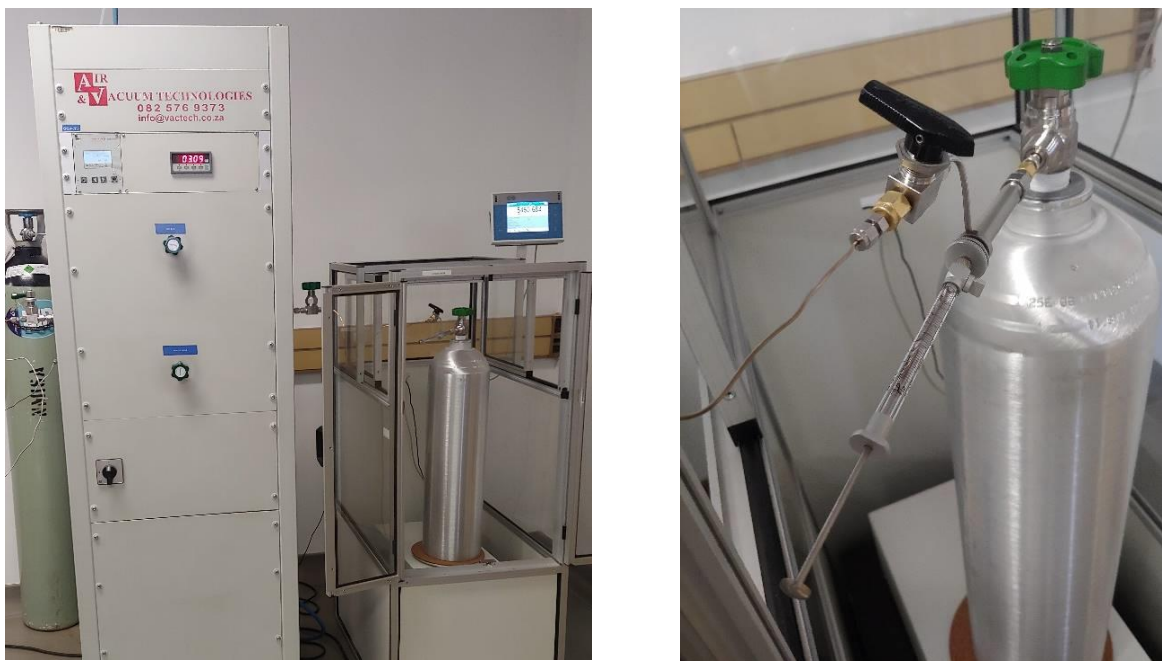
Figure 3.10: Liquid introduction system for transferring liquid sample to the cylinder
