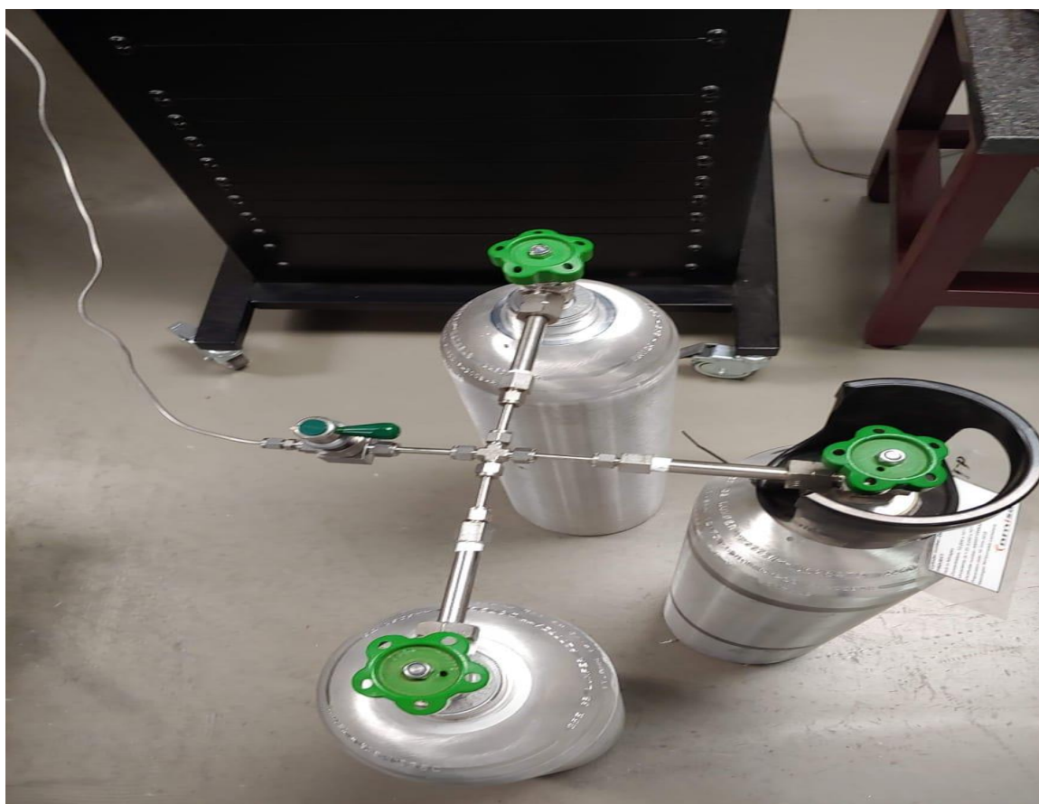
Figure 3.26: Cylinder setup for the Equal division method for adsorption/desorption test
