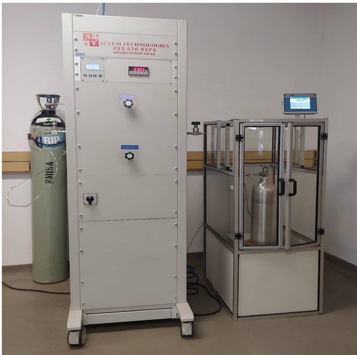
Figure 3.9: Filling station used to introduce gas components into sample cylinder
