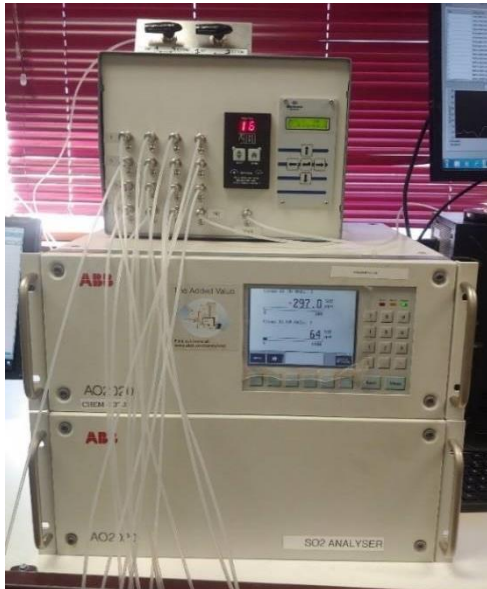
Figure 3.18: Non-Dispersive ultraviolet (NDUV) spectroscopy analysers used for analysis of hydrogen sulphide and sulphur dioxide in nitrogen primary standard gas mixtures
