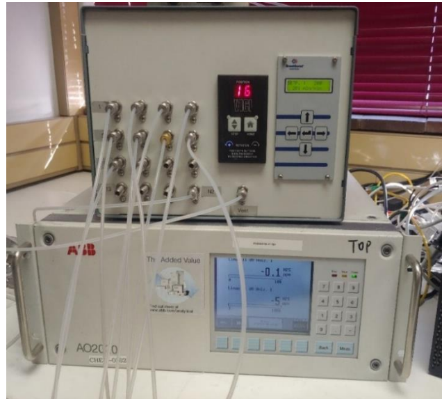
Figure 3.18: Non-Dispersive ultraviolet (NDUV) spectroscopy analysers used for analysis of hydrogen sulphide and sulphur dioxide in nitrogen primary standard gas mixtures
