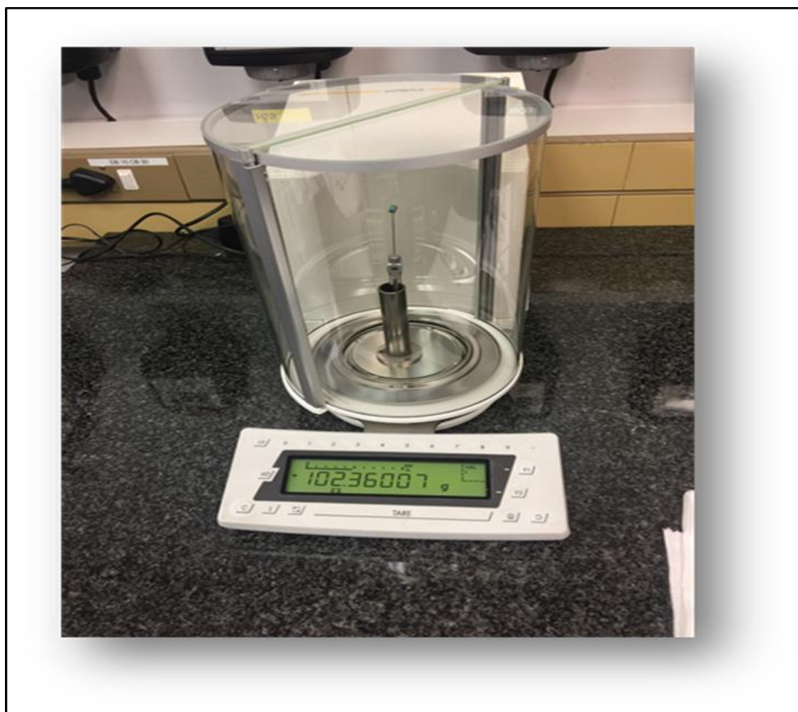
Figure 3.8: Sartorius balance used for weighing transfer vessels during the liquid preparation process.
