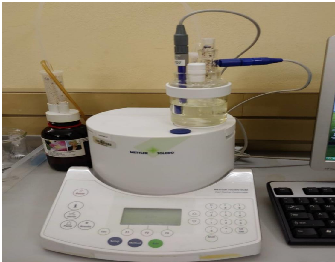
Figure 3.5: Karl Fischer titration used to analyse moisture content in high purity ethanol.
