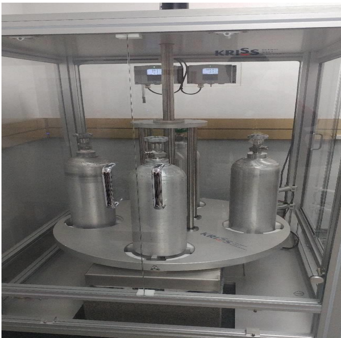
Figure 3.6: The Automatic weighing system (AWS) used to weigh cylinders on the Mettler Toledo balance.
