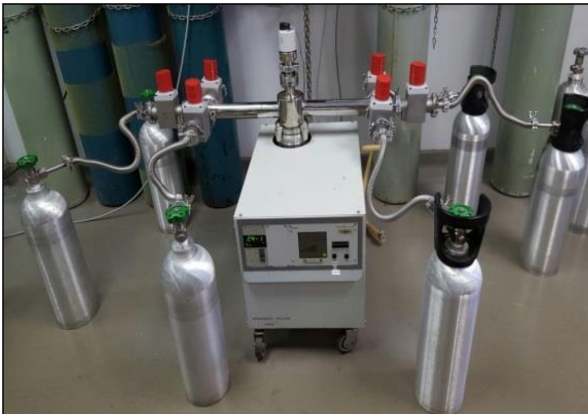
Figure 3.7: Evacuation station with a turbomolecular pump used for interior cleaning of cylinders
