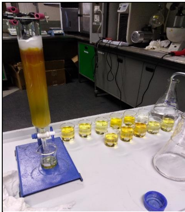
Figure 4.2: The mobile phase with approximately half the fractions already collected.
