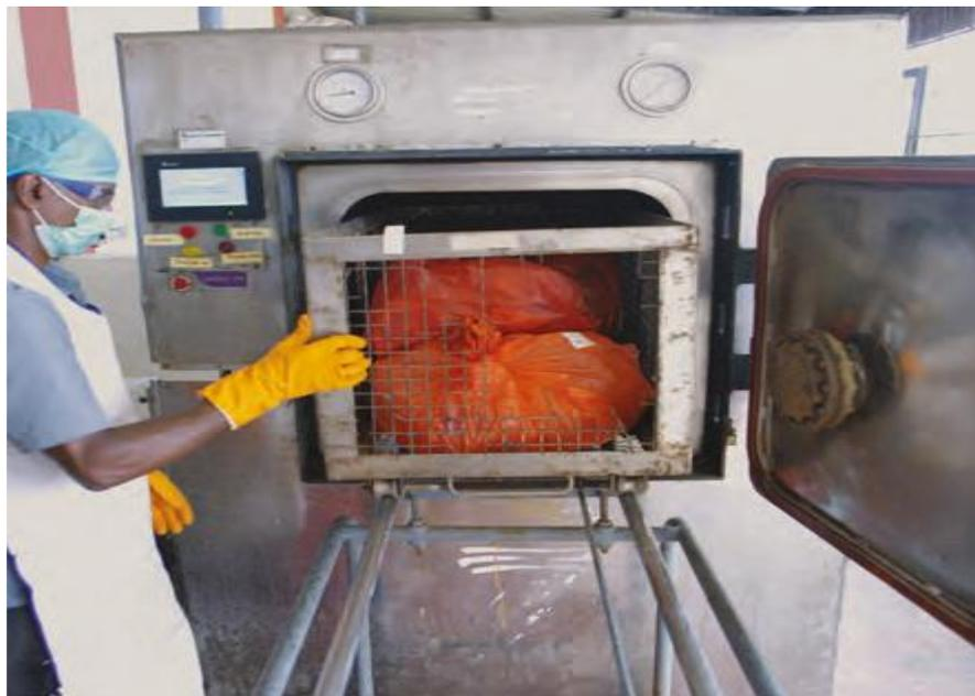
**Figure 5.24 Autoclave**
