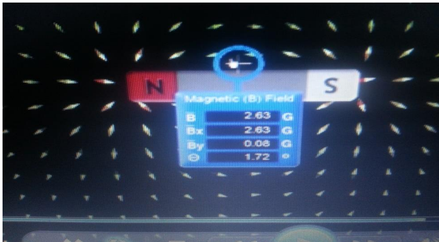
Figure 4.1 Screenshot from PhET simulations with field meter showing magnetic field strength close to a magnet
