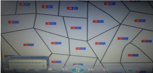
Figure 4.10 Screenshot from PhET simulations showing a magnetised material with aligned domains
