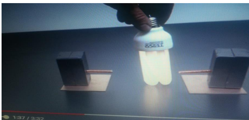
Figure 4.28 Screenshot from YouTube video showing a permanent magnet being used to generate electricity
