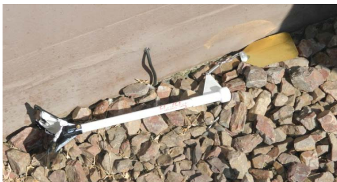
Figure 41: Fire Flag unit removed by staff members of OR Tambo building at the University of South Africa' Muckleneuk campus
