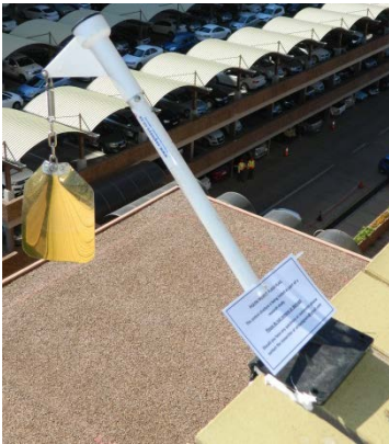
Figure 14: Flash Flag unit evaluated as a pigeon deterrent on the University of South Africa's Muckleneuk campus
