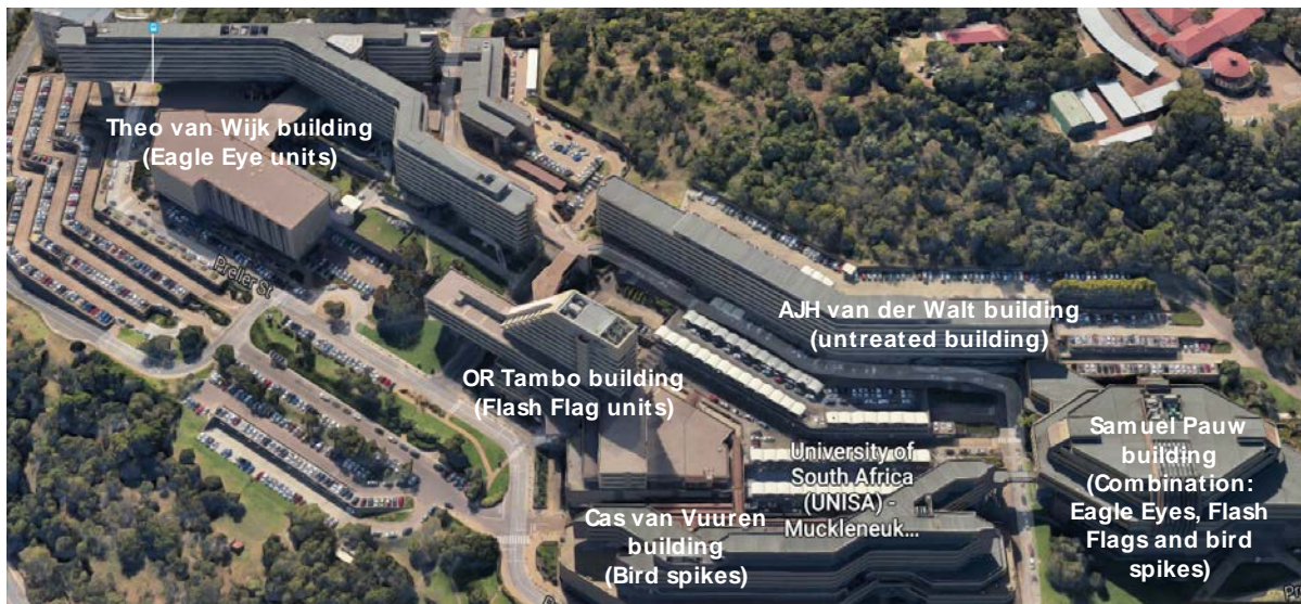
Figure 12: The University of South Africa's Muckleneuk campus in Pretoria, indicating the five buildings and their respective pigeon control structures, in proximity to each other (GoogleMaps, 2016)
