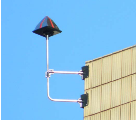
Figure 13: Eagle Eye™ unit evaluated as a pigeon deterrent on the University of South Africa's Muckleneuk campus
