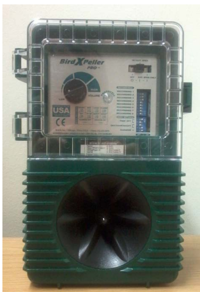
Figure 24: BirdXPeller PRO™ unit used during the implied predator presence audio trial at University of South Africa's Muckleneuk campus
