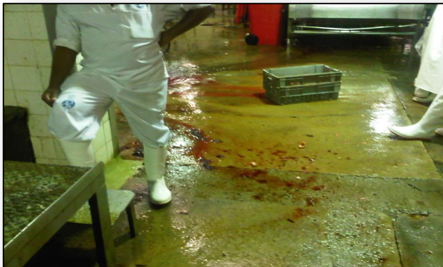
Figure 5.3 Wet contaminated floor with a cluttered floor surface. The worker is not wearing protective gloves
