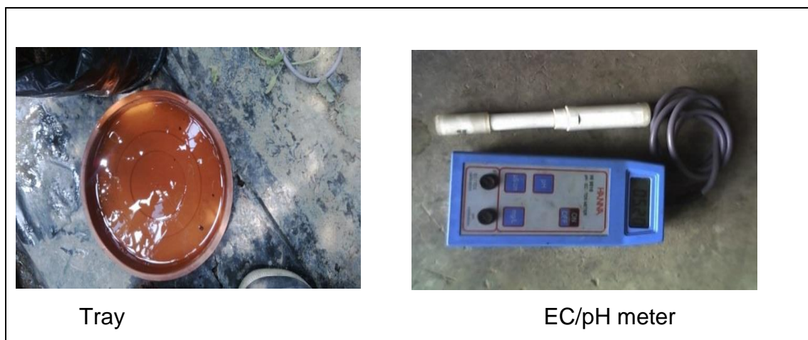
Figure 3.8 Tray used for collecting drainage water (left) and the pH meter (right).
