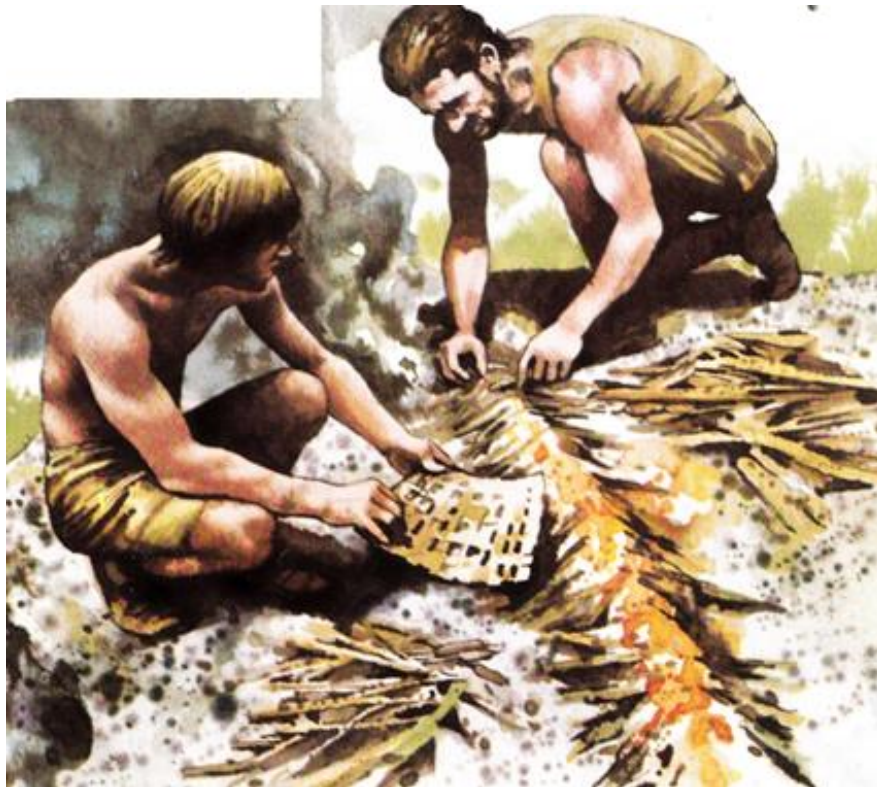
Figure 3-17: The first step in the fire setting process (Wernick 1974:123).
