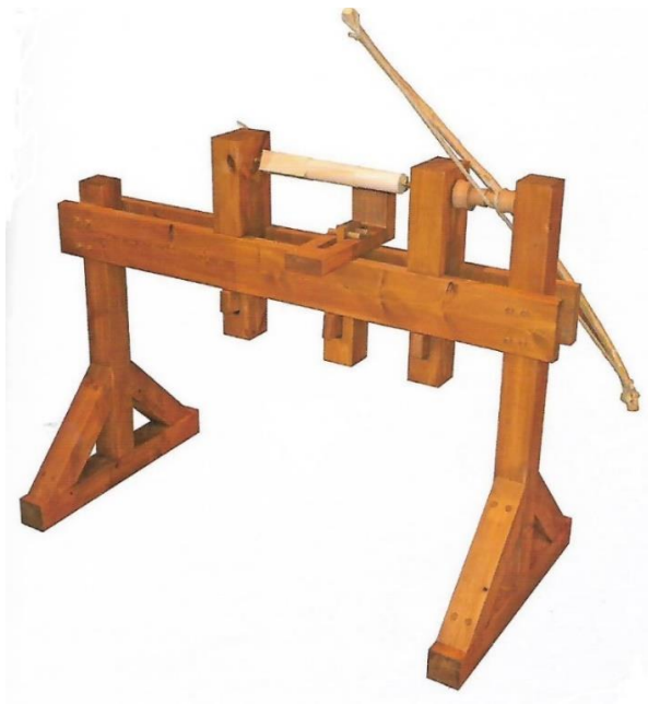
Figure 3-59: The bow lathe (Kotsanas 2017:45).
