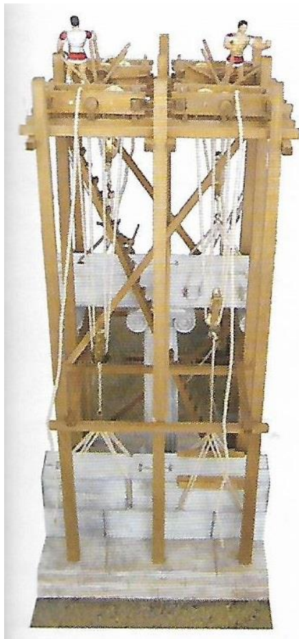
Figure 3-36: The quadpod or scaffold crane (Kotsanas 2017:97).
