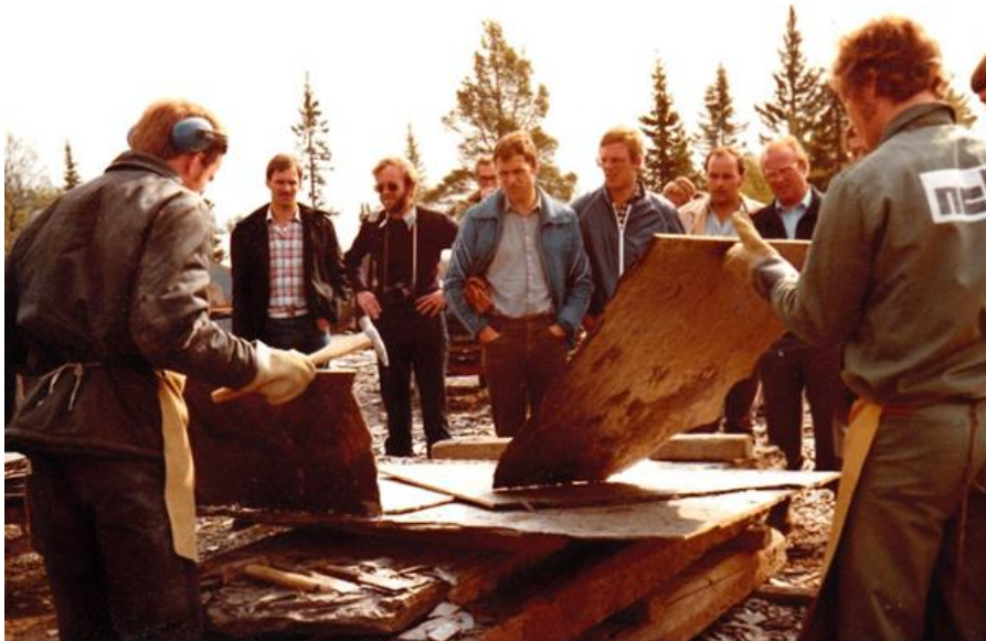
Figure 2-3: Workers splitting slate into thin layers in a slate quarry in Otta, Norway (Photograph A.M. Smith, circa 1980).
