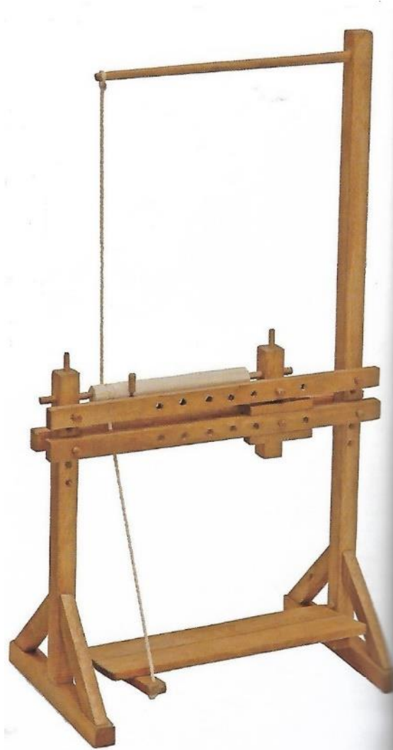
Figure 3-58: The pedal turning lathe (Kotsanas 2017:44).
