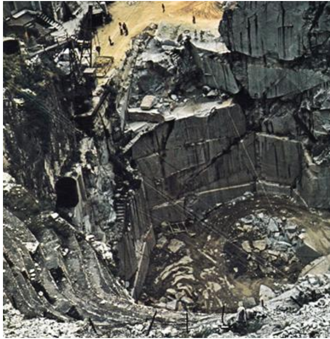
Figure 3-4: Quarry which has been worked from the top by dislodging blocks along horizontal layers, thus creating 'steps' or 'banks' as seen in the bottom left corner (Mannoni 1985:94).
