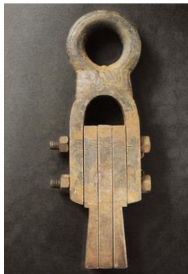
Figure 3-44: Modern version of a piece of hoisting equipment used in antiquity called a 'wolf' consisting of three metal pieces (De Nuccio & Ungaro 2002:484).
