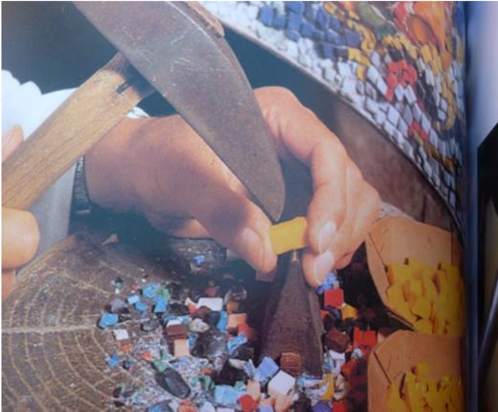
Figure 3-63: In antiquity mosaic stones were cut with the use of a hammer and small pyramid shaped anvil (Loukianós 2011:36).
