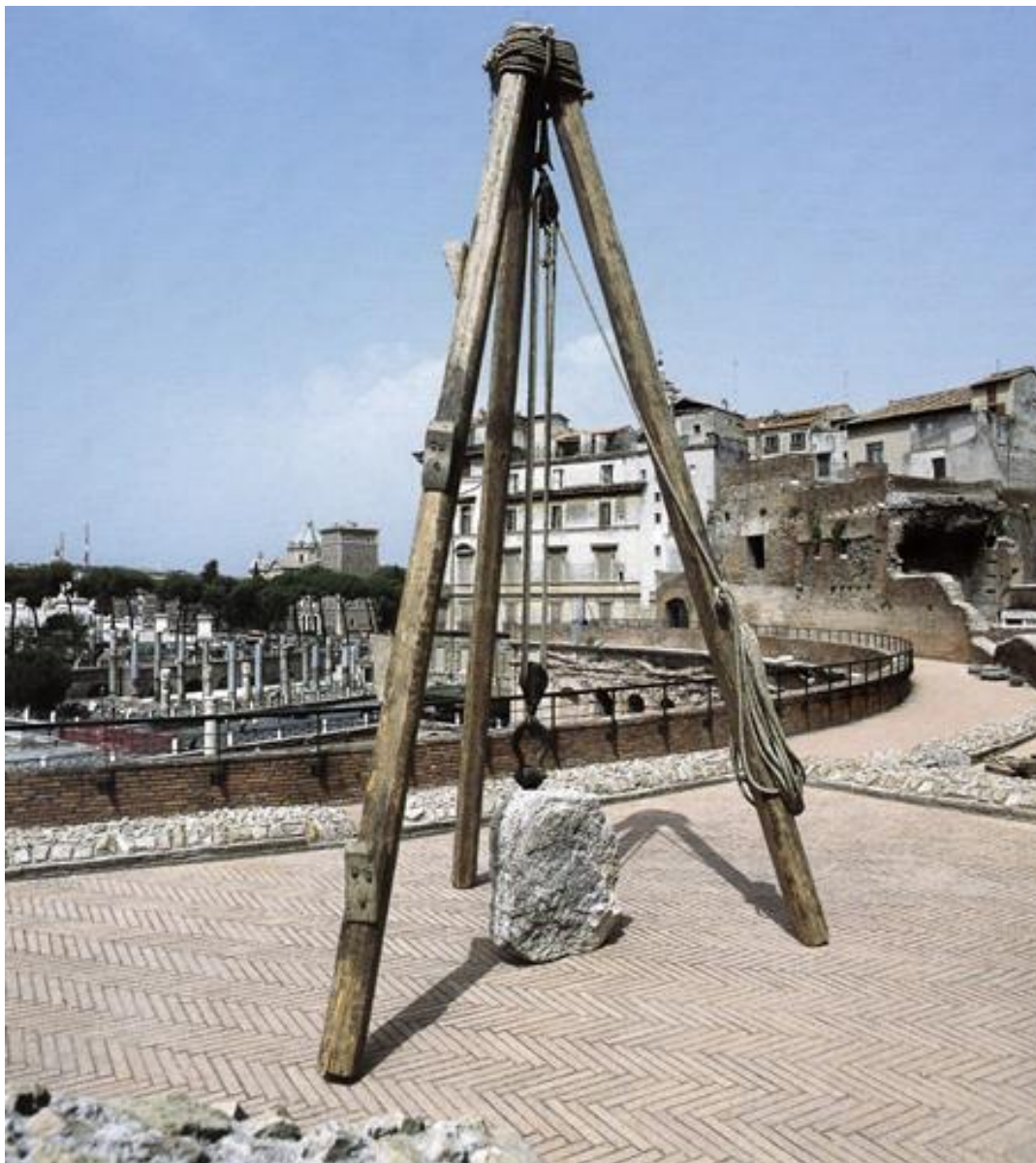
Figure 3-49: Reconstruction of a tripod crane (De Nuccio & Ungaro 2002:488).
